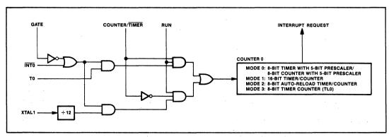
Figure 2.5.A Timer/Counter 0 Control and Status Flag Circuitry
